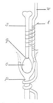
Figure 2. Grafting operation. s: style; o: ovary; p: peduncle; g: gelatine; w: iron wire; t: spider's thread (quoted from Yasuda, 1931a, b).
