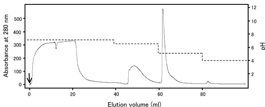
Figure 2. Profile of nickel-immobilized column chromatography. Extractions obtained with 0.5 M NaCl/50 mM Tris-HCl were performed. The amount of protein present was monitored by measuring absorbance at 280 nm. The arrow shows the application of the sample.
