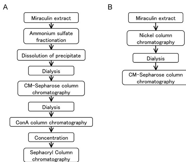
Figure 1. Comparison of purification method in previous work (A) and this work (B).
