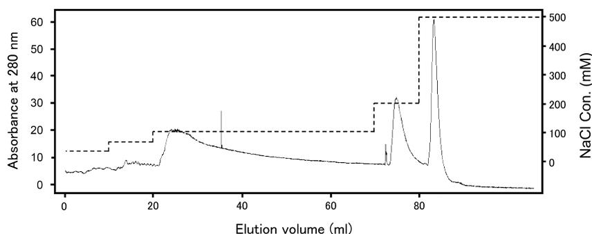
Figure 3. Elution profile of ion-exchange chromatography. The target fraction obtained from nickel-immobilized column chromatography was used. The amount of protein present was monitored by measuring absorbance at 280 nm. Elution of miraculin from the column was performed using 100 mM NaCl/0 mM Tris-HCl (pH 7.2).
