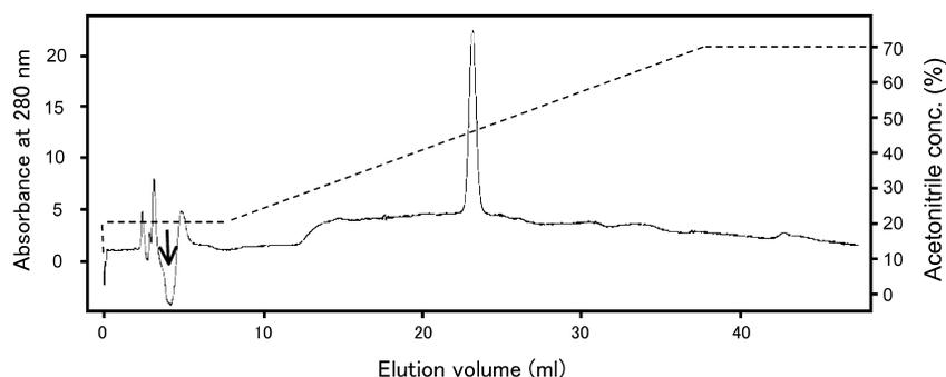
Figure 5. RP-HPLC chromatography of the target fraction. A 1 ml sample of the target fraction obtained from ion-exchange affinity chromatography was applied. The arrow shows the application of the sample.
