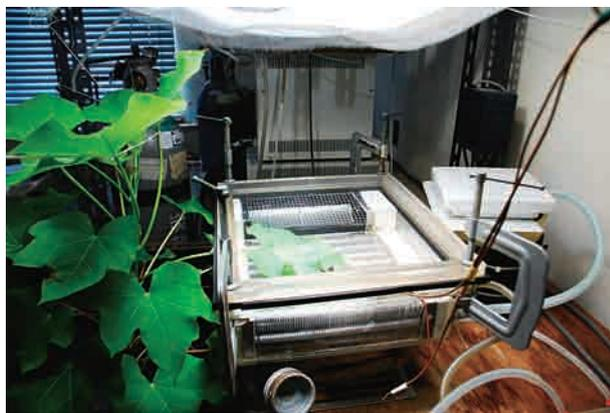
Figure 1. The CO<sub>2</sub> assimilation chamber which accommodate whole region of a leaf of *Jatropha*. The fan in the chamber eliminates boundary layer resistance and suppresses the fluctuations in CO<sub>2</sub> and humidity.
