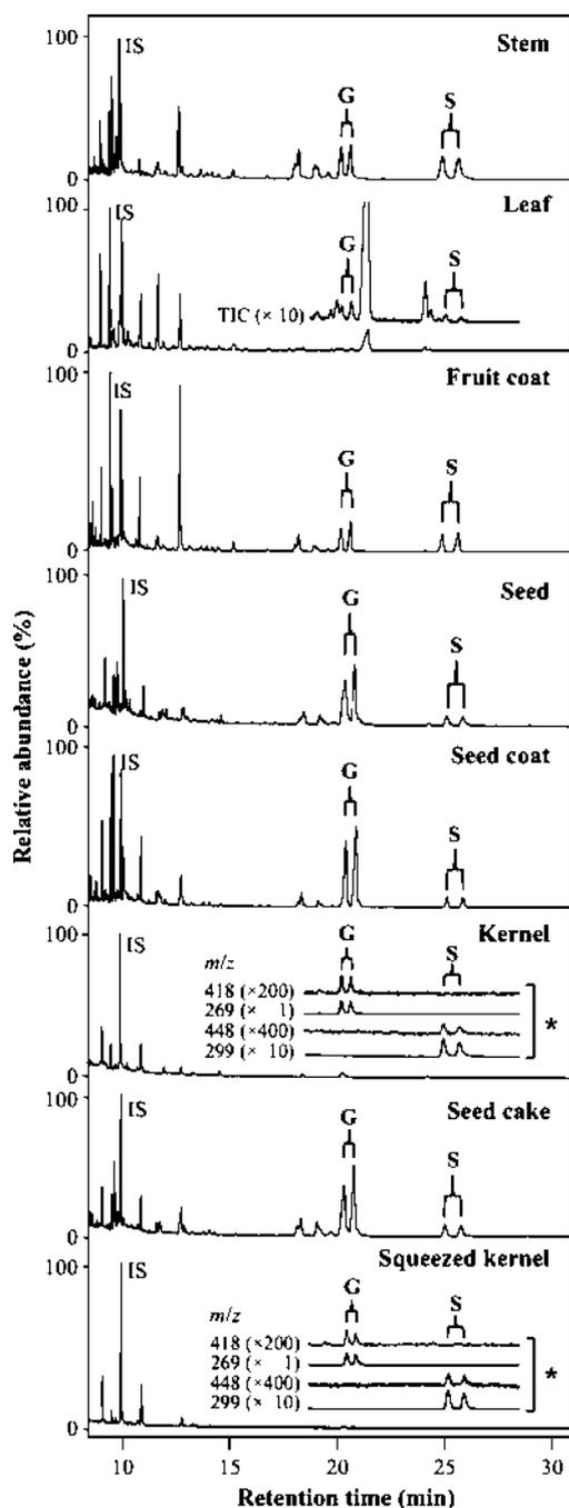
Figure 3. Total ion chromatograms of thioacidolysis products (trimethylsilyl ethers). G: guaiacyltrithioethylpropane, S: syringyltrithioethylpropane. Two peaks of G and S are *erythro* and *threo* isomers. TIC: Total ion chromatogram. \*SIM chromatogram (G:  $m/z$  418,  $[M]^+$  and base ion, 269; S:  $m/z$  448,  $[M]^+$  and base ion, 299).
