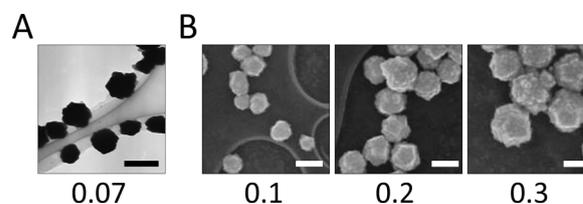
Figure 1. Micrographs of gold particles. A, TEM of  $0.07\text{-}\mu\text{m}$  gold particles; bar= $0.1\ \mu\text{m}$ . B, FE-SEM of  $0.1\text{-}$ ,  $0.2\text{-}$ , and  $0.3\text{-}\mu\text{m}$  gold particles; bars= $0.2\ \mu\text{m}$ .
