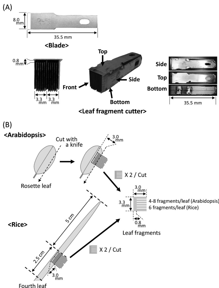
Figure 1. Structure of the leaf cutter and the images of cutting leaves. (A) Structure of the leaf cutter. (B) Scheme for the preparation of *Arabidopsis* and rice leaf fragments.
